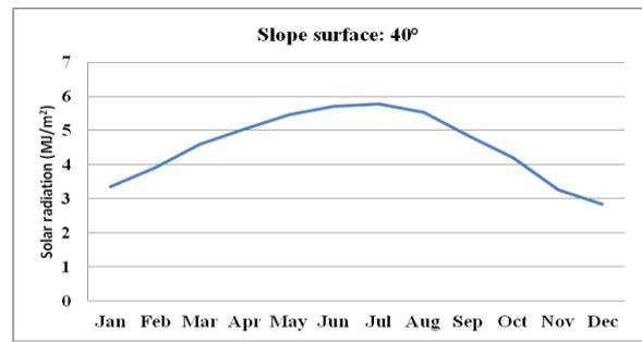
Figure 3. Solar radiation on tilted surface
